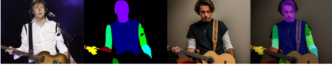
FIGURE 4.2: Conditional image generation from DensePose. Left to right: original image, estimated DensePose using [Güler, Neverova, and Kokkinos, 2018], generation from estimated DensePose, overlay of the generated image with its control
