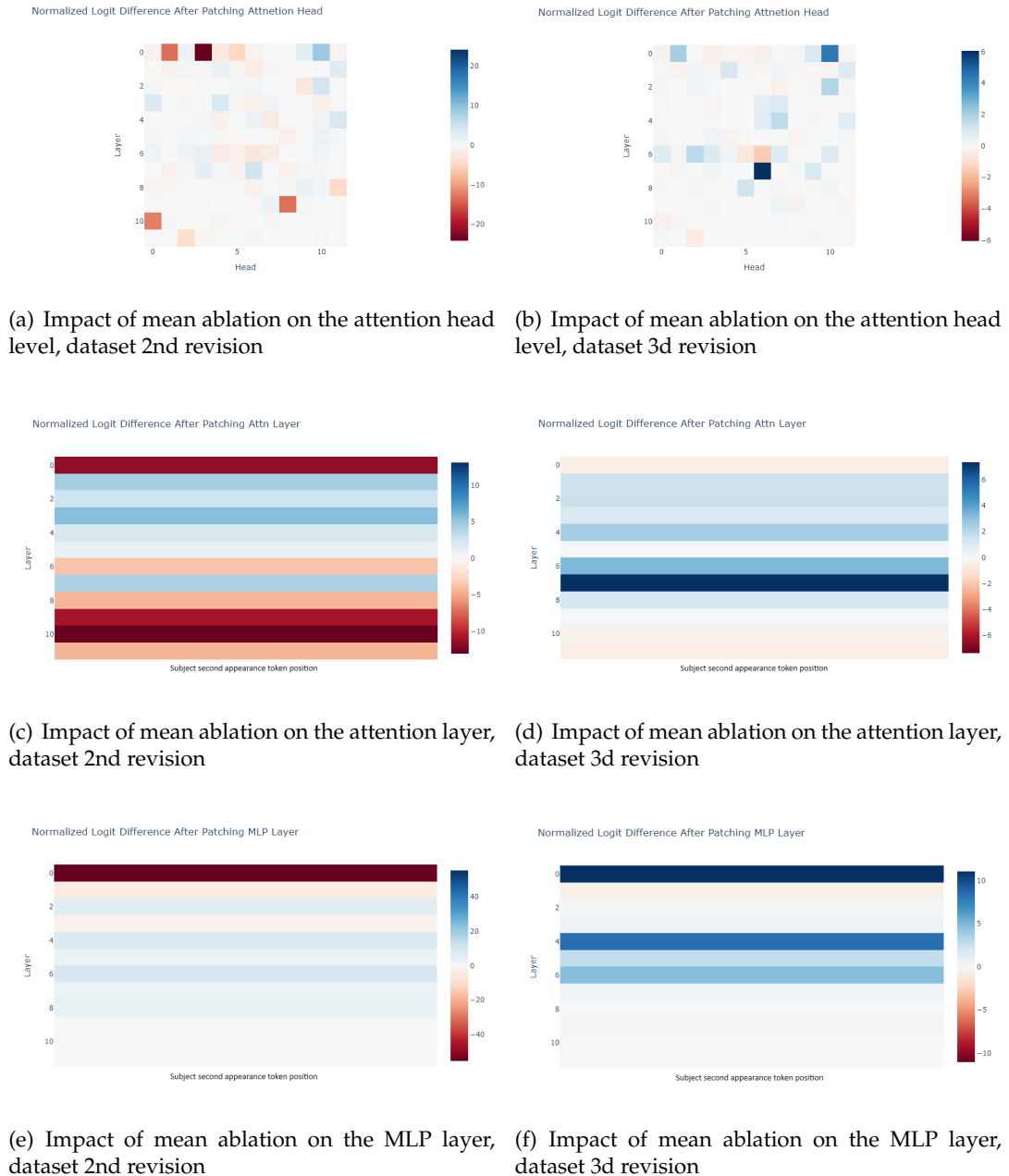
FIGURE 5.7: 1st experiment. Mean ablation done on GPT-2-small, comparison between 2nd dataset revision (left column) and 3d dataset revision (right column) on the subject second appearance token position . Figures show the indirect effect on output probability mapped for the contribution of (a, b) attention head, (c, d) only attention activations, (e, f) only MLP activations.
