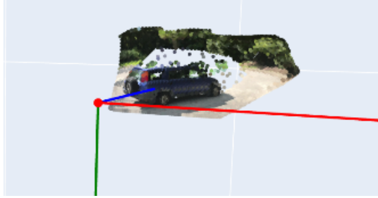
FIGURE 5.1: Unprojected pcd in camera space for I_0 frame car sequence. Here axes represent camera orientation with blue being forward, red is right and green is up vectors.
