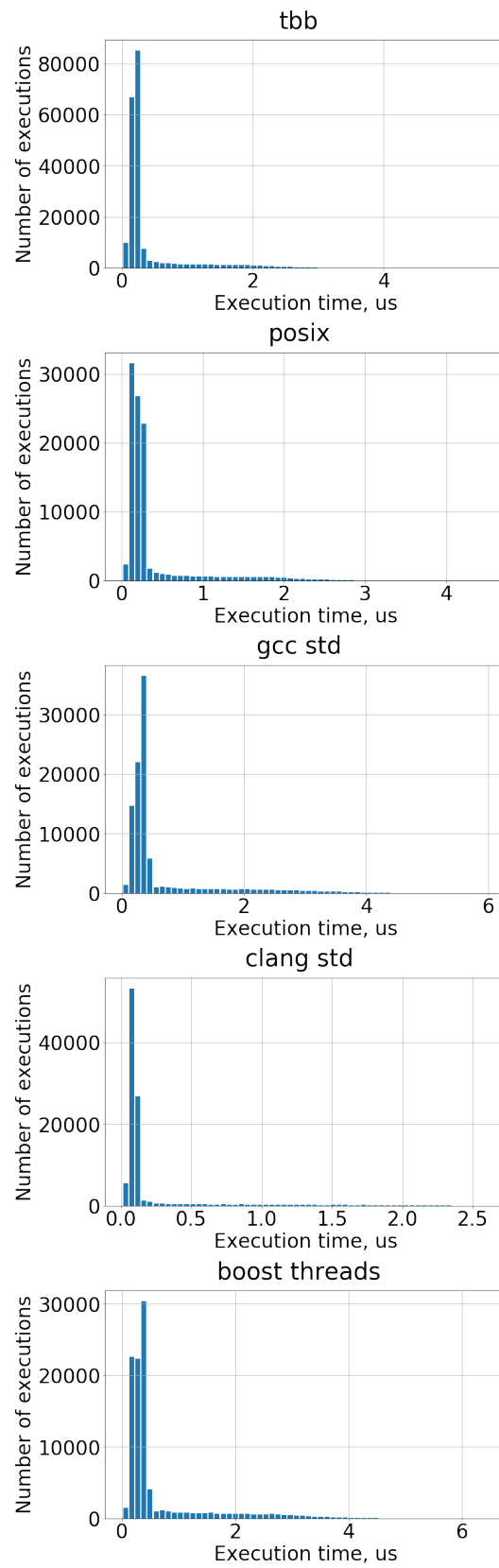
FIGURE A.5: Histograms of the received time results of same mutex request per one iteration by thread when creating 100 threads in one program on HP Probook 440 G5.
