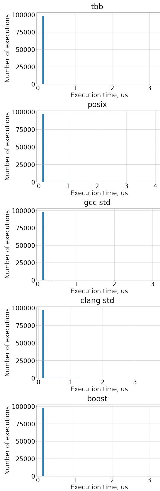
FIGURE A.6: Histograms of the received time results of same mutex request per one iteration by thread when creating 100 threads in one program on Raspberry Pi 3.
