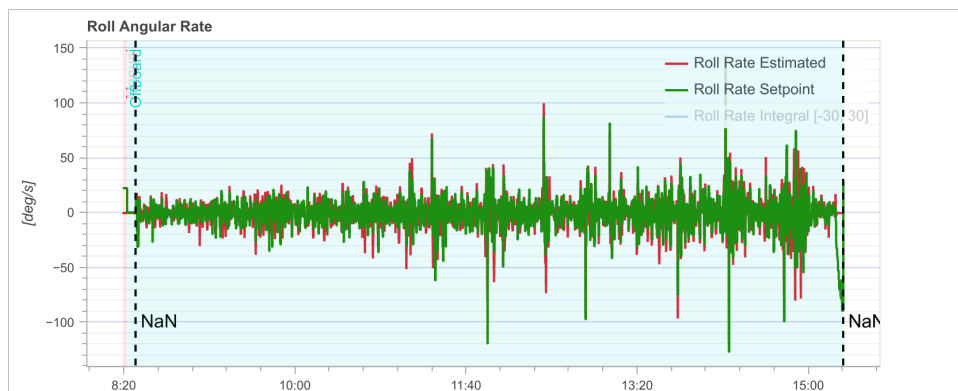
FIGURE 5.7: Roll rate response from Pixhawk4 during real flight.
