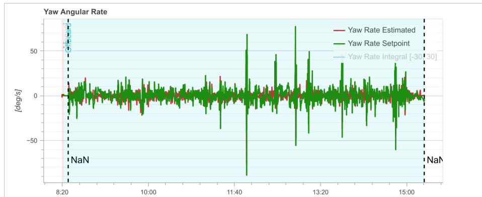
FIGURE 5.5: Yaw rate response from Pixhawk4 during real flight.
