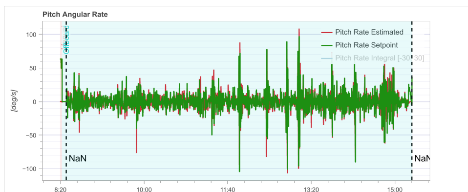
FIGURE 5.6: Pitch rate response from Pixhawk4 during real flight.
