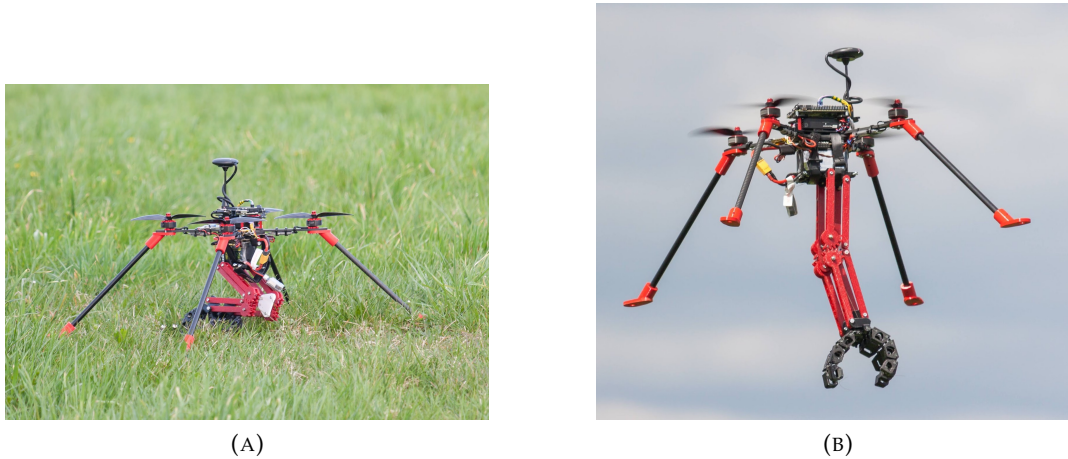
FIGURE 5.4: UAV in real-world testing. (A) Landed state, legs bent; (B) Legs unbent during flight 4 .
