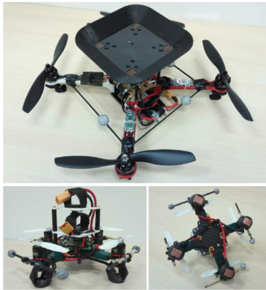
FIGURE 3.2: Top: Main UAV with the docking platform and spring-loaded connectors. Bottom: Flying battery with docking legs and copper plate connectors. Taken from [6].
