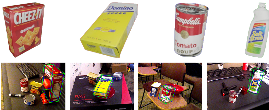
FIGURE 5.4: Pose Detection Examples. The green cuboid in images represents the ground-truth object pose. The blue cuboid represents the predicted object pose.
