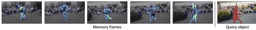
FIGURE 2.3: Memory bank readout operation. The multiple frames are kept in memory bank covering different object poses, scales and backgrounds. For the query (i.e. current) frame visual features are matched with visual features stored in memory and the best correspondence is selected. The most important features for the query object are shown as bright regions on memory frames. Image taken from [22].
