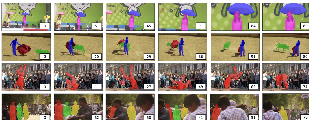
FIGURE 2.1: Semi-supervised Video Object Segmentation formulation. For the first frame segmentation masks for some object instances are given. The target is to correctly predict the segmentation masks for all the following frames. Challenging scenarios typically include: similar objects (rows 1, 3, 4), complex occlusions (rows 2, 4), drastic scale (row 1) and shape (rows 2, 3) change. Image taken from [22].
