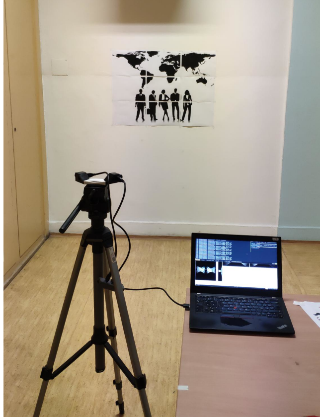
FIGURE 5.1: The setup for experiments. The designed prototype is located on a tripod, at distance d from the plane \Omega with visual features. The with Y - Z plane of the cameras' common coordinate frame is parallel with \Omega . A set of 9 A4 papers with features was used to make \Omega distinguishable.
