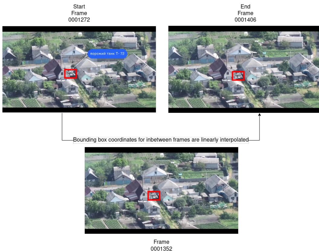
FIGURE 3.4: Annotator manually positions bounding boxes in the start and end frames. All frames between the two are linearly interpolated
