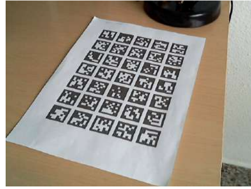
(B) ArUco board OpenCV: Detection of ArUco Markers 2023
