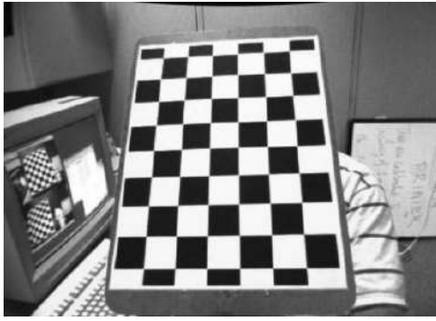
(A) Chessboard OpenCV: Camera Calibration 2023
