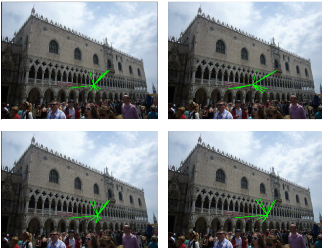
FIGURE 5.2: Visualisation of self-attention for points that belong to a single repeated texture at the first layer in AGNN. For each keypoint in repetition only top 10 attention weights are shown as lines between query and key. Keypoints from the same repetition attend to very similar set of keys independent of their position.
