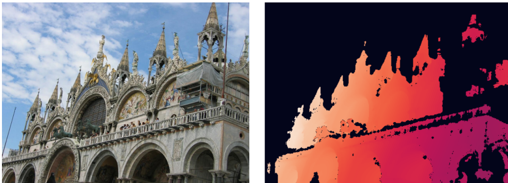
FIGURE 5.1: Example of the image (left) and corresponding depth map (right) from MegaDepth dataset. Brighter values in the depth map represent larger depth values. Missing depth information is shown in black.
