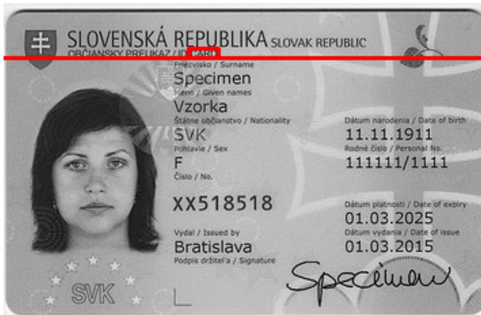
FIGURE 4.1: Position of "CARD" in a bounding box. The part above the red line should be removed
