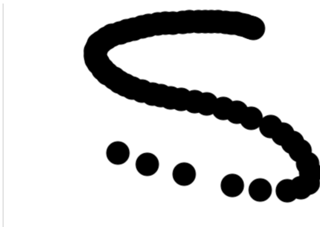
FIGURE 3.5: The "brush" tool core idea: stamp-like drawing on every mousemove event fired.
