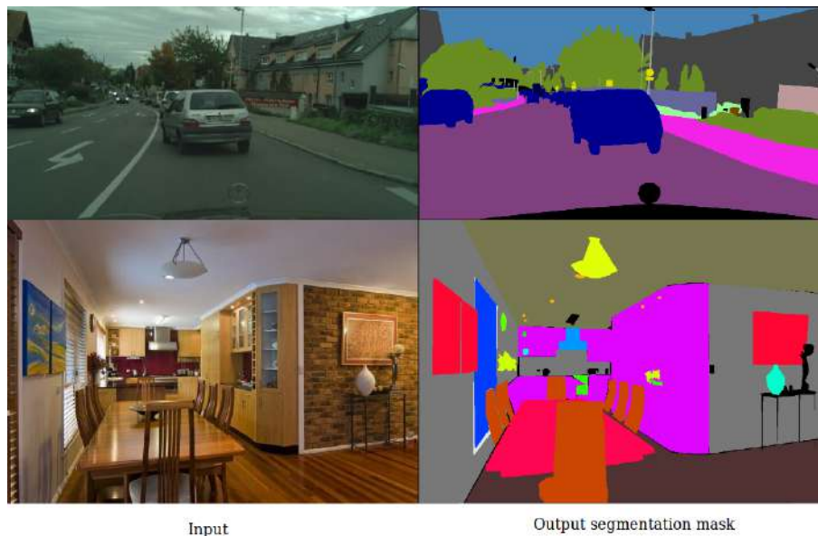
FIGURE 1.1: An illustration of the scene semantic segmentation task. In the input we take some scene (on the left), and produce the output semantic segmentation mask for a scene (on the right). The images are taken from Cityscapes [6] and ADE20K [30] datasets.
