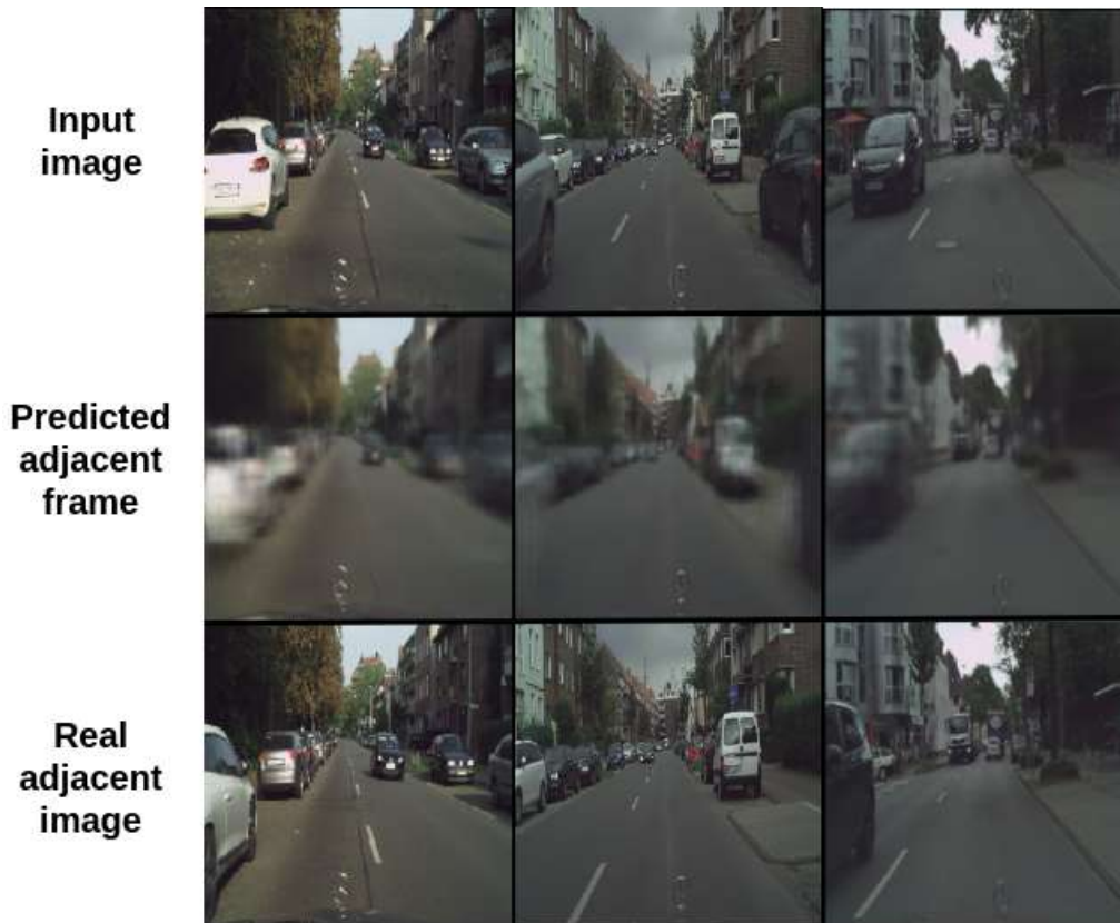
FIGURE 3.4: Examples of images being produced by the generator. Objects (cars) which are close to camera and situated from the sides are expected to partially disappear from the following frames, respectively blurred or distorted by generator.
